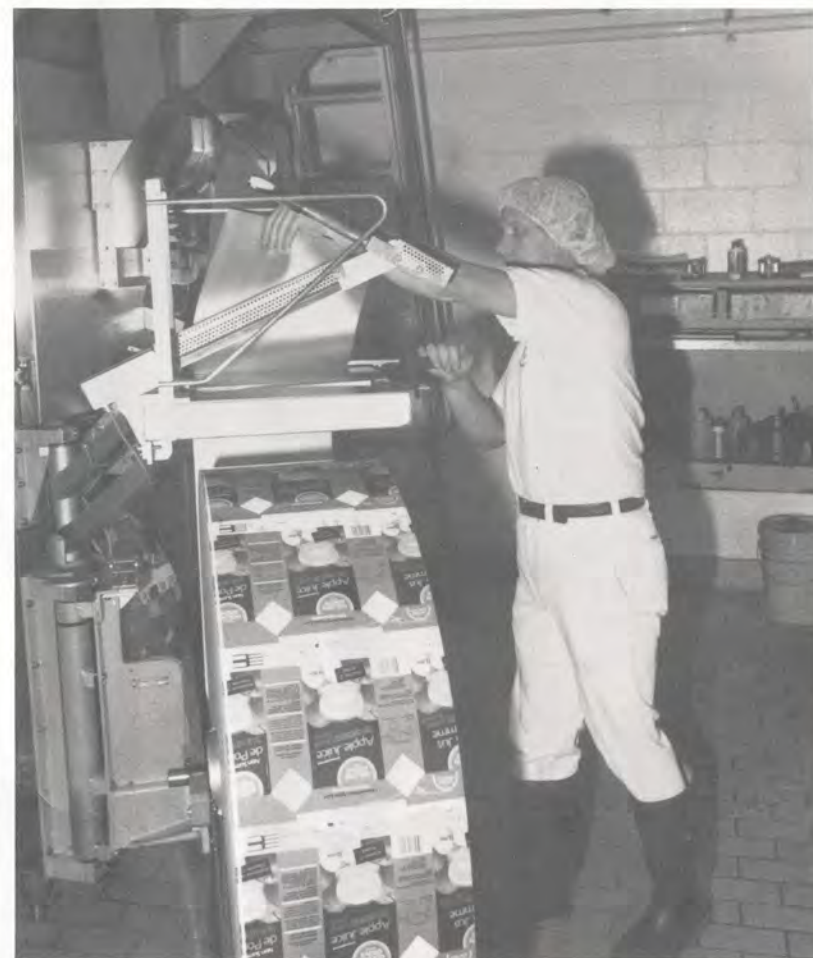
Holiday relief dairy worker/packager Terry Bunke splices paper rolls together on the one litre filler at the Annacis plant.
