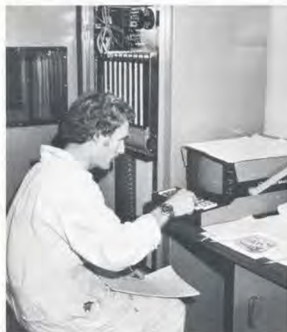
Dick Rice of Burnaby's maintenance department, learns to operate the new Programmable Controller which will control all processes on the production floor.
