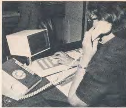
As customer orders are phoned in, the operator types the product code and quantity on the keyboard of the terminal. This relays the information directly into the main computer.
