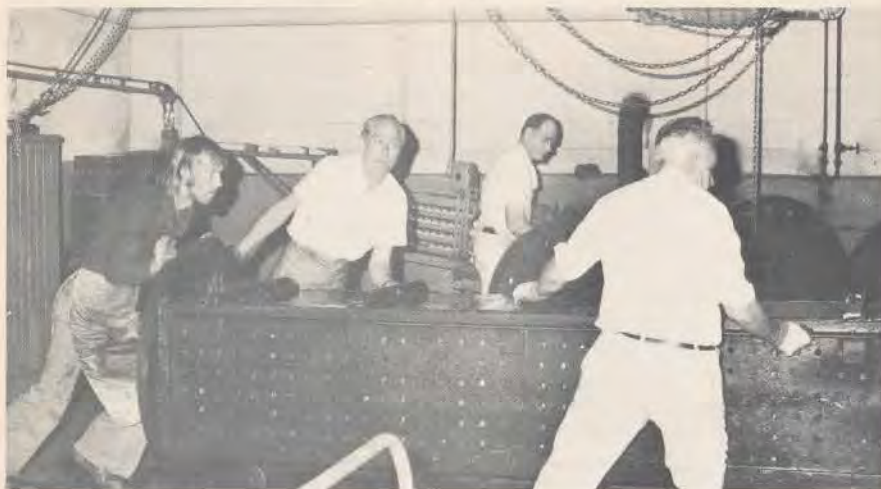
Removing cages from the Pacific Milk midget retort (sterilizing chamber) are (l-r) LES HENDY, KEN BLOOMFIELD, REUBEN BAERG and PETE DEJONG.
