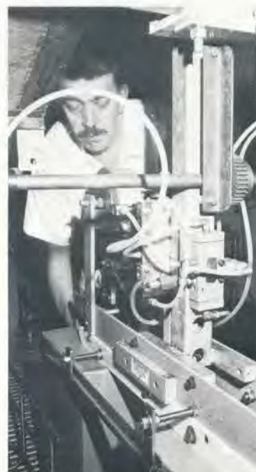
Strong poly tape, top and bottom, now seals bulk milk cases cleanly and efficiently. This new system replaces a gluing process which was difficult to handle and required many hours of maintenance. DAN FLEMING, Plant Maintenance Foreman, investigated the problem and selected the equipment. The operator here is BILL GAUNT.
