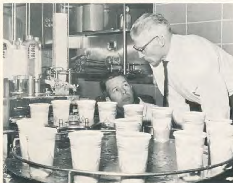
BARRY CRANE and LARRY SHAW inspect new yogurt filler. The machine is filling 60 cups per minute now and the speed could be increased for future demands to 180-190 cups per minute. The entire cost of the filler was $11,000, including labour.
