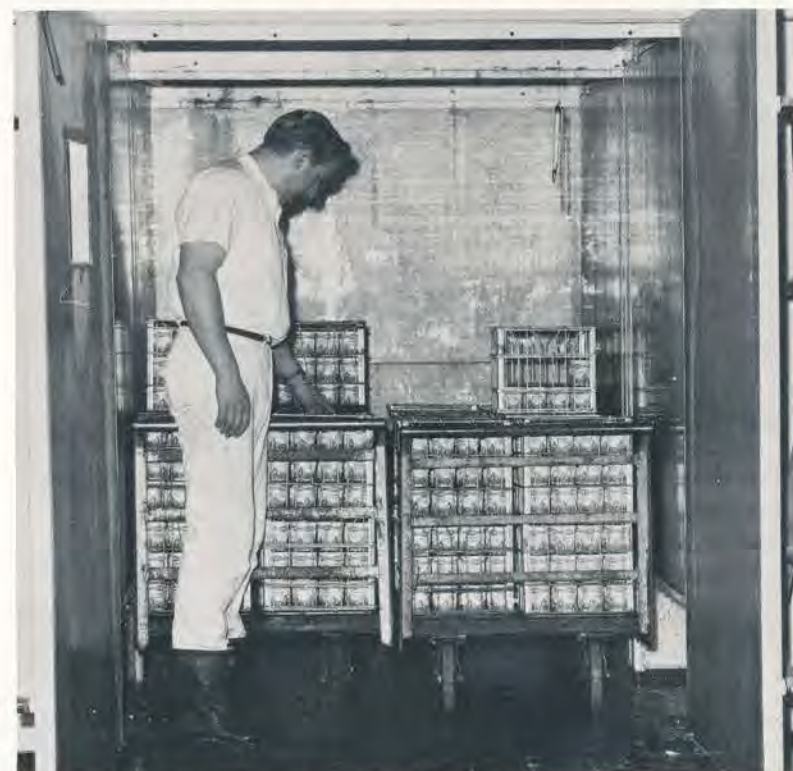
KAL PEDERSEN, Dairyland special products maker, checks a batch of yogurt in the Burnaby plant's new incubator. The walk-in unit, brought from Holland, was installed in the room where the sour cream and yogurt is prepared. With the incubator, Dairyland can more than double the current capacity now produced. It also permits a higher degree of quality control on yogurt which Dairyland markets in a variety of flavors. About 700 pounds of yogurt is being incubated during each setting.
