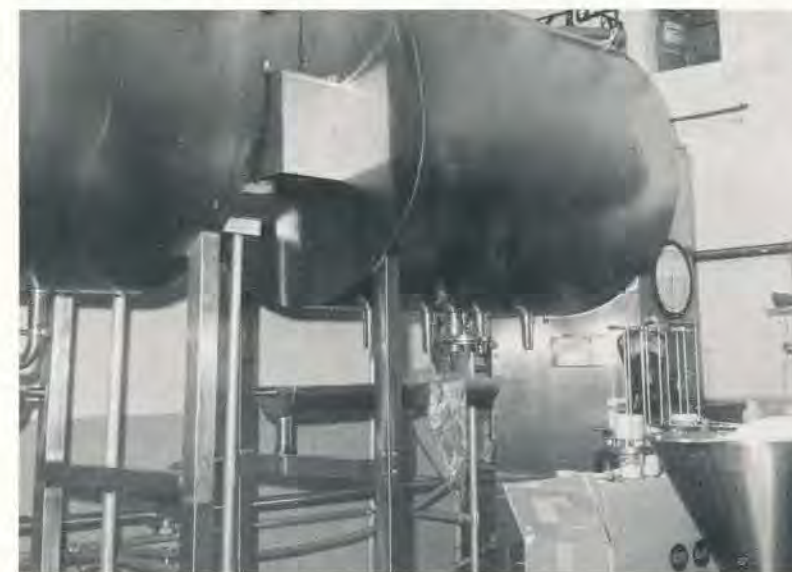
THESE TWO GRACE MIXERS have added a new dimension to the production of cottage cheese at Sardis. They will drain the curd, mix in the dressing, store the curd overnight and give an accurate measurement of the amount of cheese they hold.
