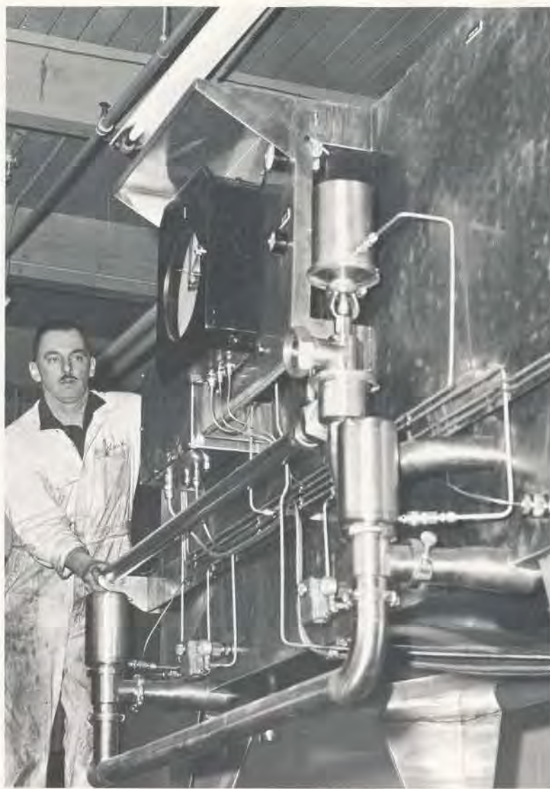
DON LAND of the Burnaby maintenance shop swings a new Cleaned-In-Place washing unit out to the loading dock. The unit is being installed at the Abbotsford plant where it will do the cleaning in milk tank trucks, plant tanks and plant lines. Aside from the tank, the CIP unit was built entirely in the FVMFA's Burnaby shops.
