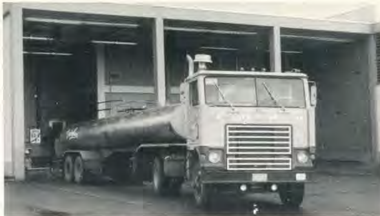
DAIRYLAND'S TRUCK FLEET is expanded by the latest purchase of a Tandem Axel Tractor. A WT 1000 D Ford with a 335 engine, the new tractor will be large enough to carry a load of 55,000 pounds of milk, considerably more than the vehicles presently used. A new semi trailer tank is also on order and this combination of tractor-trailer will accommodate the maximum gross vehicle weight.
