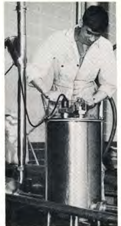
Per Nielsen puts the finishing touches on a level control tank he constructed in the workshop. This tank keeps a constant flow on the flow meter when milk is pumped into the holding tanks from tank trucks.
