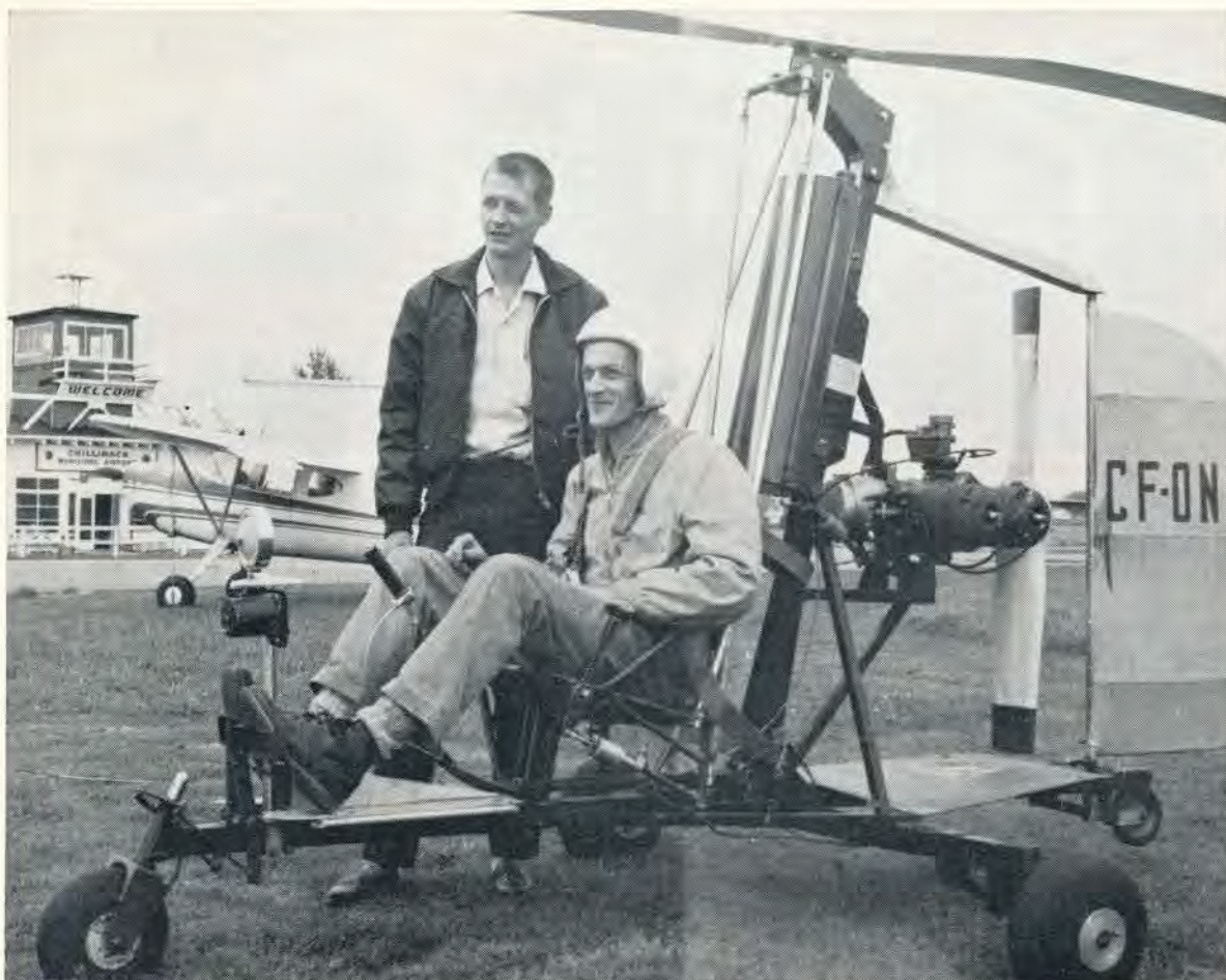
SUCCESSFUL TEST RUNS over, Ron Montie poses with his home-made autogiro at Chilliwack airport. At the controls is John Edmeston who was piloting the craft when it crashed at Delta Air Show, after the smaller driving propeller behind him suddenly disintegrated.
