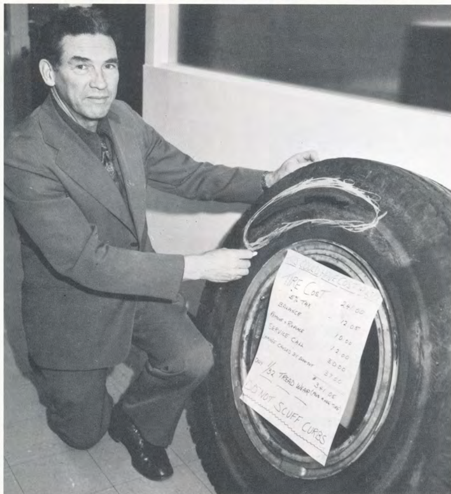
Mel Hand, Wholesale Supervisor, demonstrates what could have caused a serious accident. As our driver stopped at a small store account, this tire blew out with such a force that it broke one of the store's windows. The wall of the tire had been weakened by continual scraping against curbs. Fortunately the driver was not on the highway when this happened.
