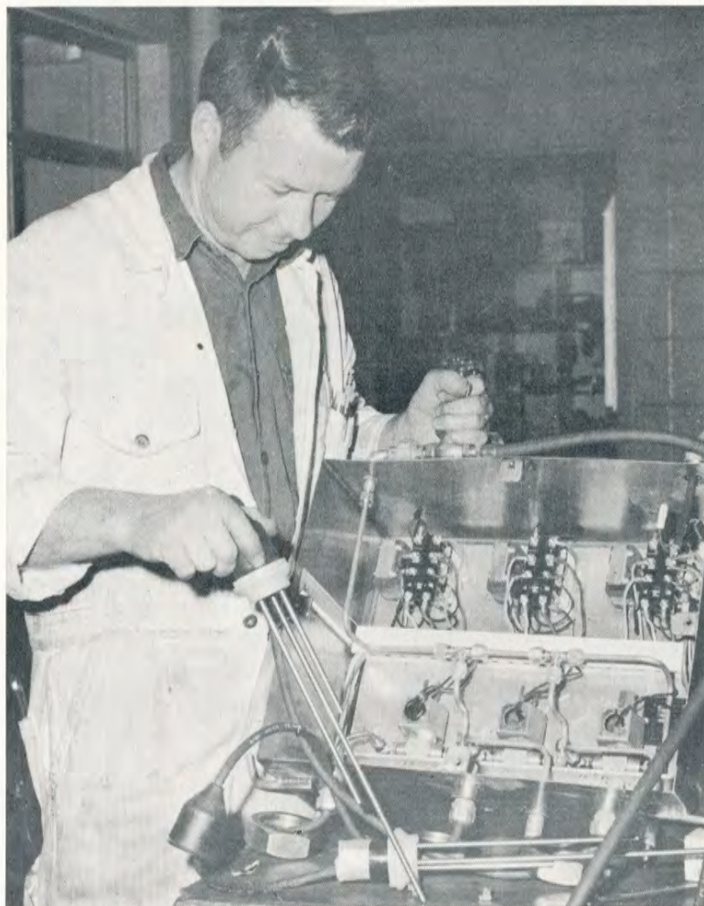
Level controls that automate the liquid flow in the Vita-line are checked by maintenance man Barry Craine. The equipment was designed by Plant Maintenance Supervisor Larry Shaw. It was made in the Burnaby plant's workshop.
