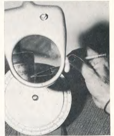
The markings on the "tach" discs are checked to see how long a stop is taken at a farm tank pickup.
