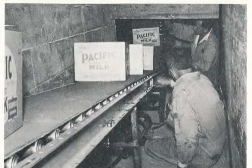
Fred Gillberg and Fred Goldsmith make adjustments to the new conveyor system. The cases of canned milk leave the production floor of the Abbotsford plant, slip under the railway tracks before moving upwards into the holding warehouse.
