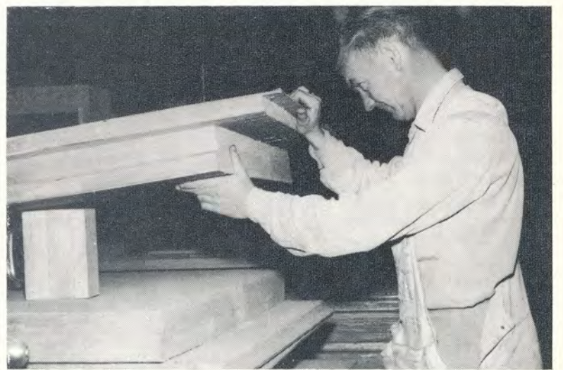
JACK PHILLIPS in the Burnaby plant's carpentry shop checks one of the pre-fabricated panels that makes up the low temperature cold room at the Terrace depot. Final fitting adjustments were completed by erecting the room here.
