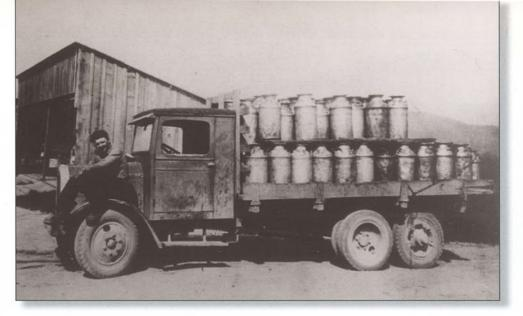
Wesley Simpson leaning against one of his family's International Harvester trucks used for milk pick-up. This truck had a pony axle behind the drive axle and hauled double-decked ten-gallon cans to the FVMPA's Sardis utility plant or to the Borden plant in South Sumas. Undated.
